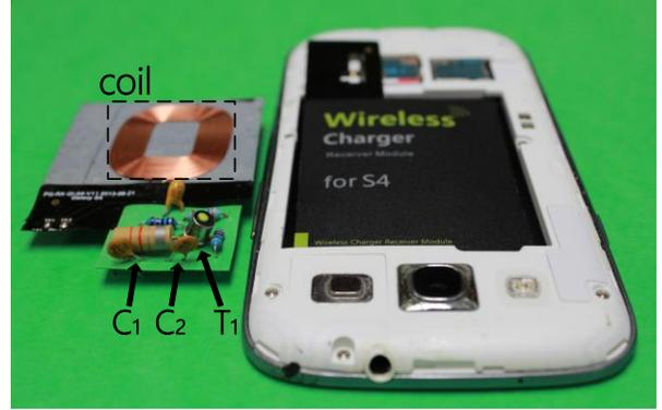
Fig. 3. The off-the-shelf wireless power transfer coil for non-contact interaction with the phone, the coil and the customer designed driving circuit.
