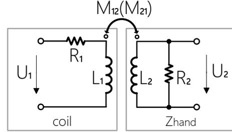
Fig. 1. Circuit model of inductive non-contact interaction.
