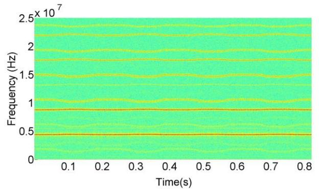
Fig. 4. Short-time FFT of resonant waveform when hand movement is performed in front of the inductive coil.
