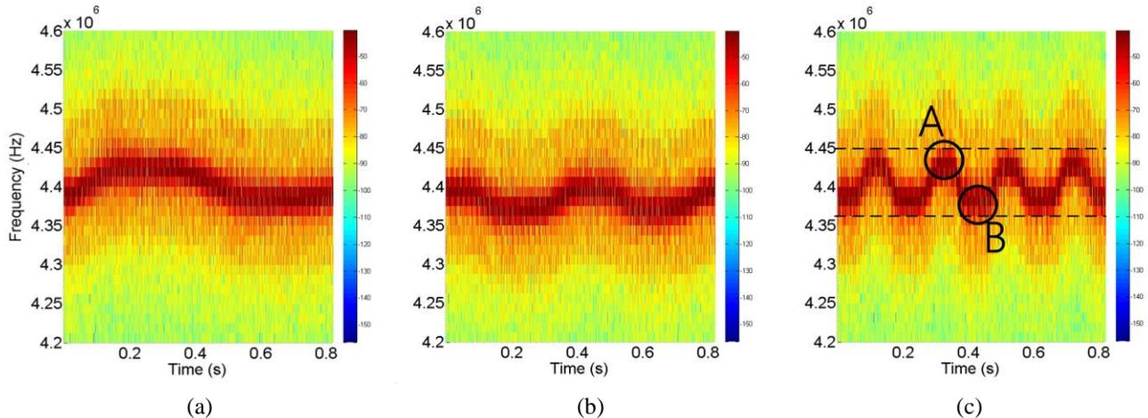
Fig. 5. Zoom-in view around fundamental resonant frequency of the coil. (a), (b) and (c) show how resonant frequency changes when different hand movement (waved one, twice and three times, respectively) is performed in front of the coil in 0.8 second.
