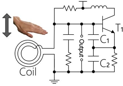
Fig. 2. Oscillator circuit with inductive coil.
